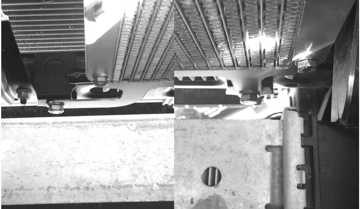
Lower Transmission Cooler Mounts, center on left, outer on right
