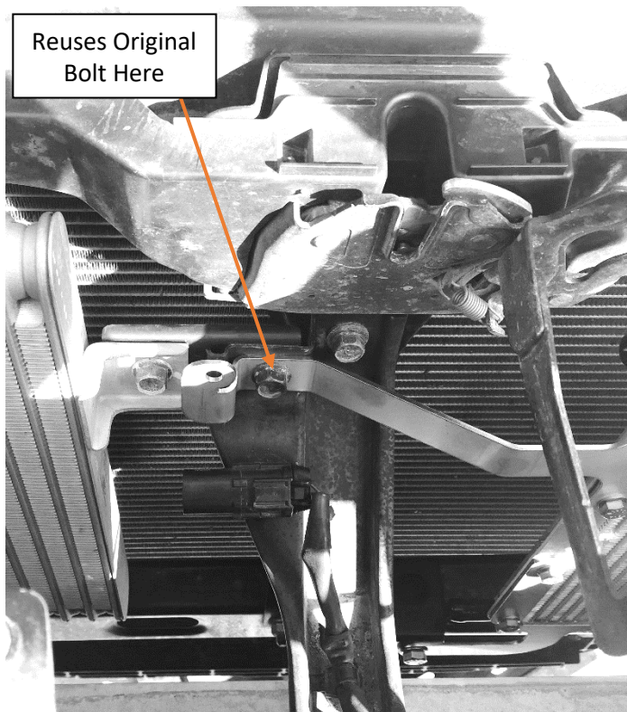
Top Center and Top Outer Transmission Cooler Mount
