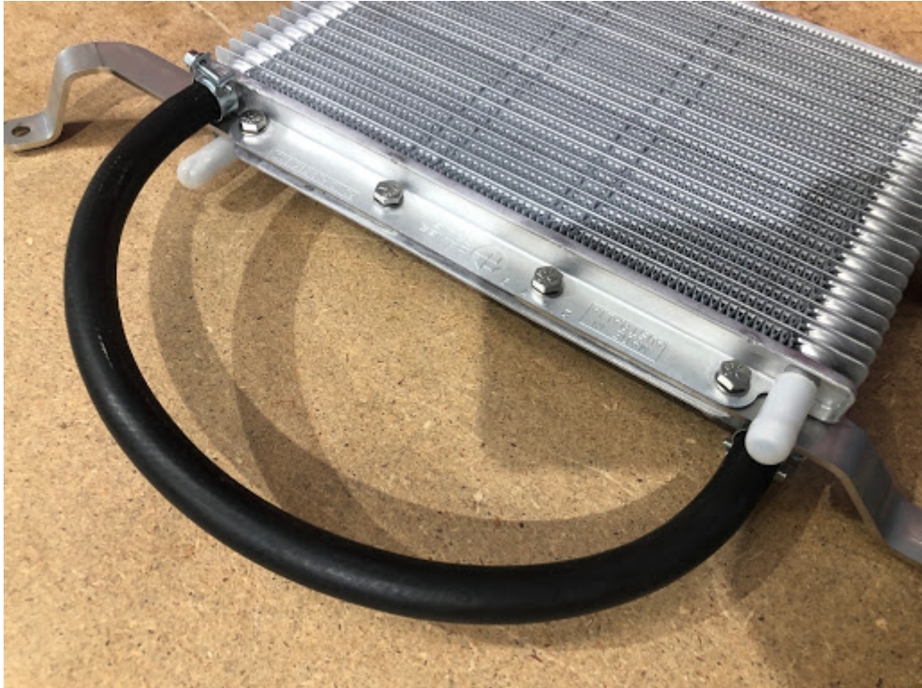
Image shows dual cooler mounting and hose connection
