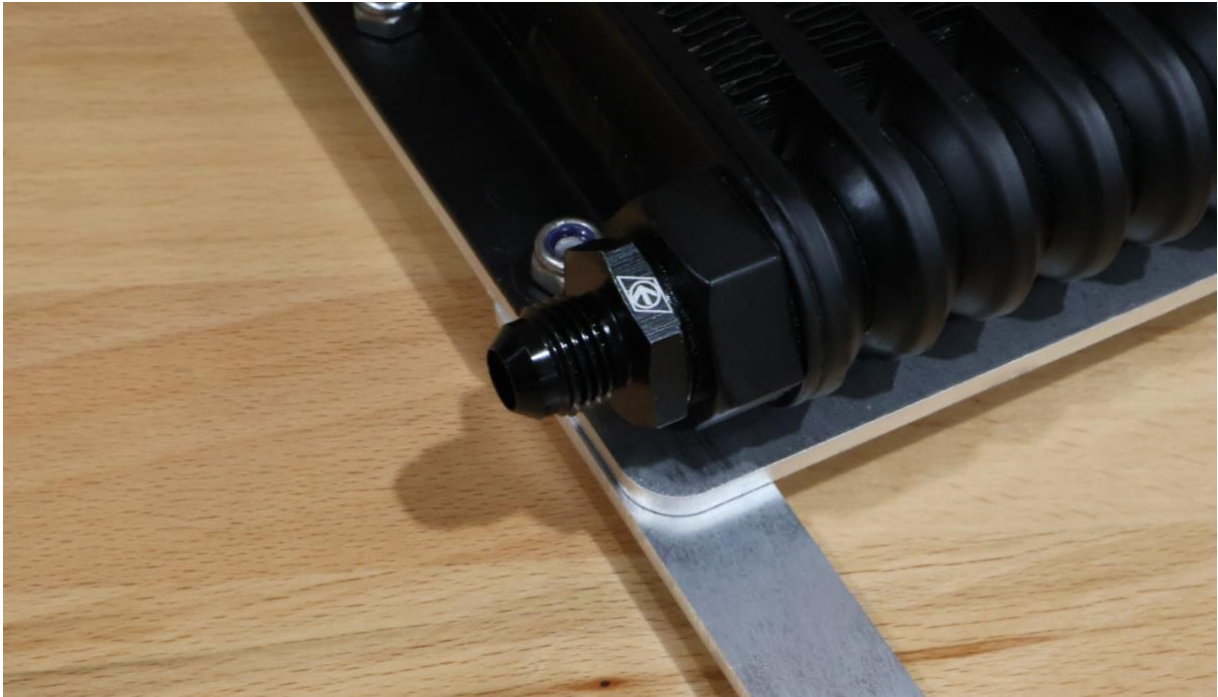
M16x1.5 adaptor and alloy washer secured to cooler with Loctite 567
