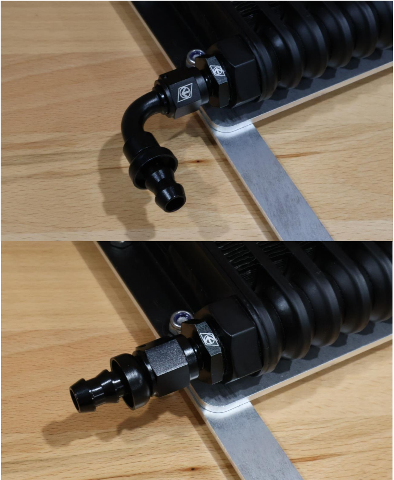
Examples of straight and 90° hose tails installed on M16x1.5 to -6 adaptors.
