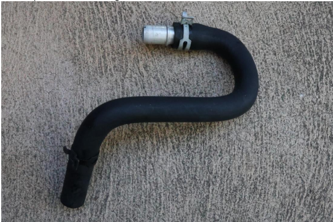
New coolant hose prepared with original clamps and new coolant adaptor fitting.
