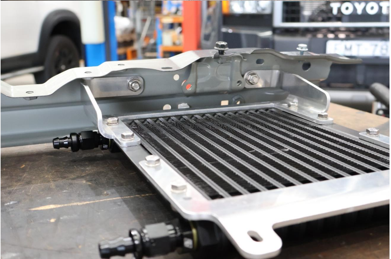
Transmission Cooler Assembly Secured to Radiator Support Crossmember (hoses not installed)
