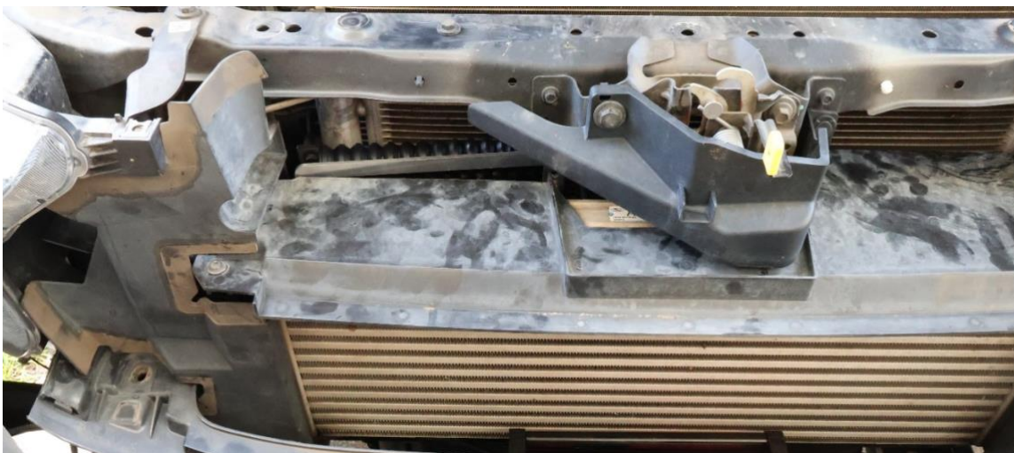
Intercooler and trim pieces reassembled.
