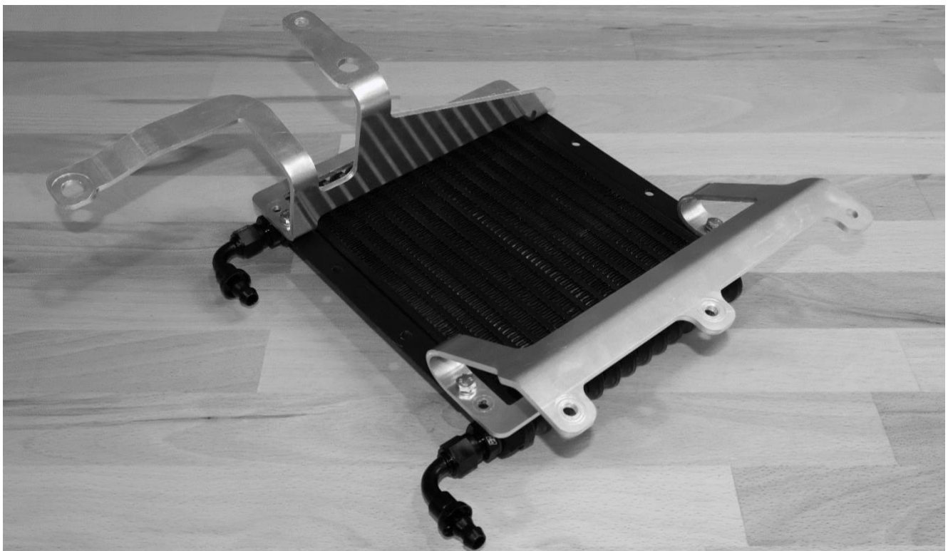
Cooler assembly with fittings in place at correct orientation
