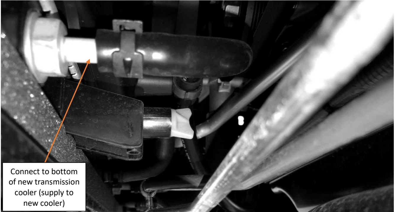
Version 1 Stock transmission cooler lines in lower radiator tank.
