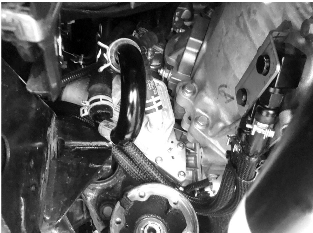
Transmission cooler lines in place to new transmission adaptor block, note drive shaft removed for clearer photos
