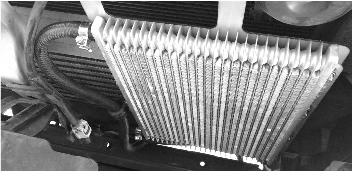
Make sure hose does not rub on center support
