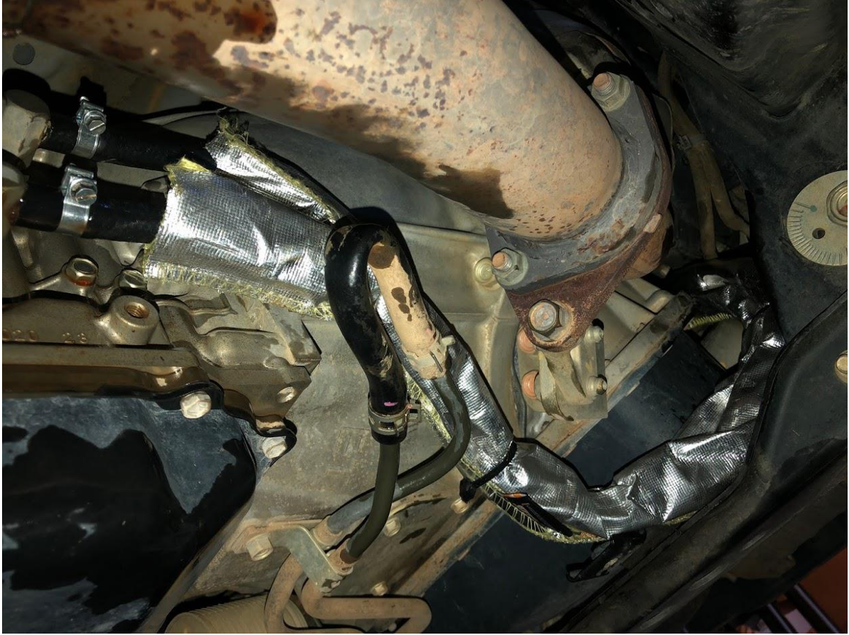
Route the hose away from the exhaust when securing
