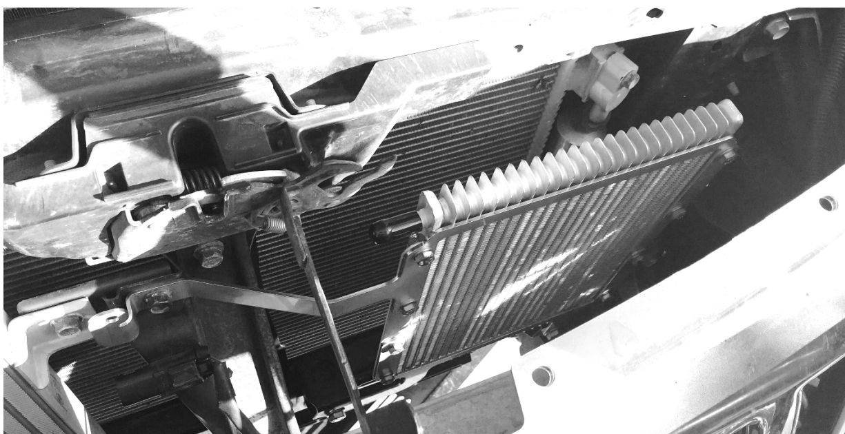
Transmission Cooler Assembly Bolted in Place. Note: Cooler sits on rear face of brackets, with nuts towards the rear, bolts to the front.
