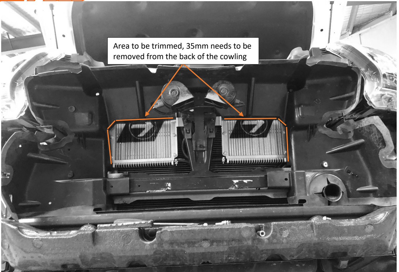
Example of trimmed cowling for Everest fitment, if only one cooler is fitted only one side needs to be trimmed
