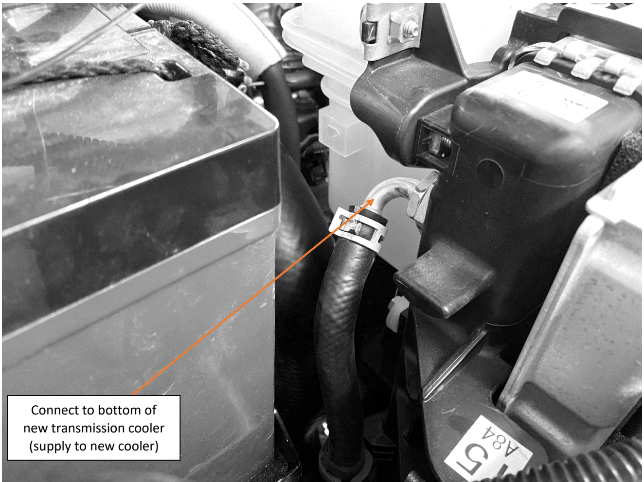
Version 2 Stock transmission cooler lines in driver's side radiator end tank
