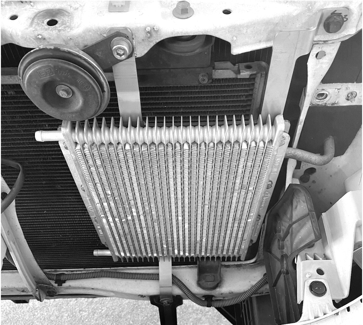
Transmission Cooler Assembly Bolted in Place. Note: Cooler sits on front face of brackets, with nuts towards the rear, bolts to the front.
