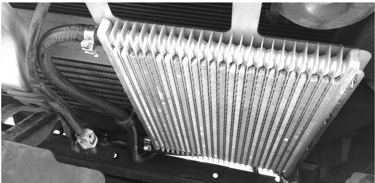
P Clip Bolted in Place. Make sure hose does not rub on center support
