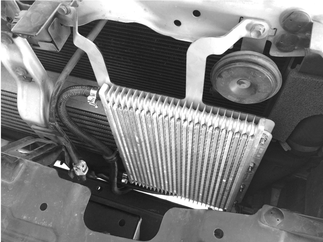
Transmission Cooler Assembly Bolted in Place. Note: Cooler sits on front face of brackets, with nuts towards the front, bolts to the rear.
