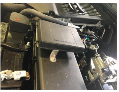
3. Install the STEINBAUER Power Module to the vehicle. Once the module is installed and the harness is attached to the module place the module onto the bracket, using zip ties attach the module to the bracket.
