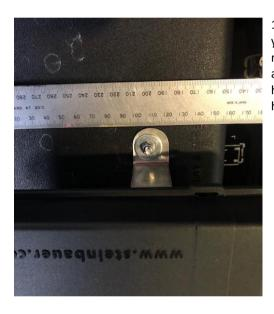
1. Remove the fuse box cover, hold the bracket in place so you can get a rough idea of the mounting location. Place some masking tape on the top of the cover where the top leg sits and along the face closest to the engine. Measuring from the right hand top edge, place a mark at 110mm, this is the center of the hole for the top leg.
