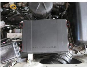
5. Feed the Steinbauer harness up through the mounting bracket. Clip the Steinbauer harness onto the module. Run the harness along the engine bay, using Zip ties to secure the harness away from any hot or sharp surfaces. Connect the module onto the injector drivers following the Steinbauer module instructions. Check the function of the LED light on the module. Once completed use Zip ties to secure the module to the bracket in each corner of the module as pictured.
