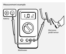
Measure the voltage with a multimeter on the plug-in connection
