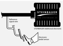
Solder the reference signal wire on the wire of the electronic pedal sensor.
