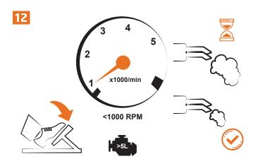
Allow the engine to idle until most of the smoke has stopped.
