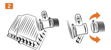
Locate the air intake pipe and disconnect the hose after the MAF sensor if fitted to your car.
