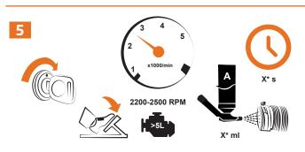
Hold the engine at 2200 to 2500 RPM while the first shot of 250ml (A) is sprayed into the air intake.
