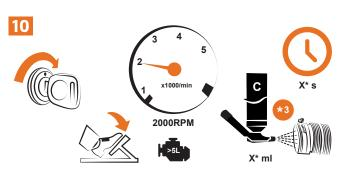
Start the engine, bring it to 2000 RPM then apply the third 250ml (C) shot into the air intake.
