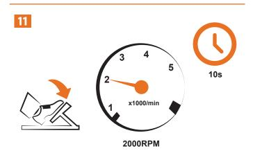
Hold the engine at 2000 RPM for 10 seconds.
