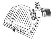
Re-attach the intake pipe.
