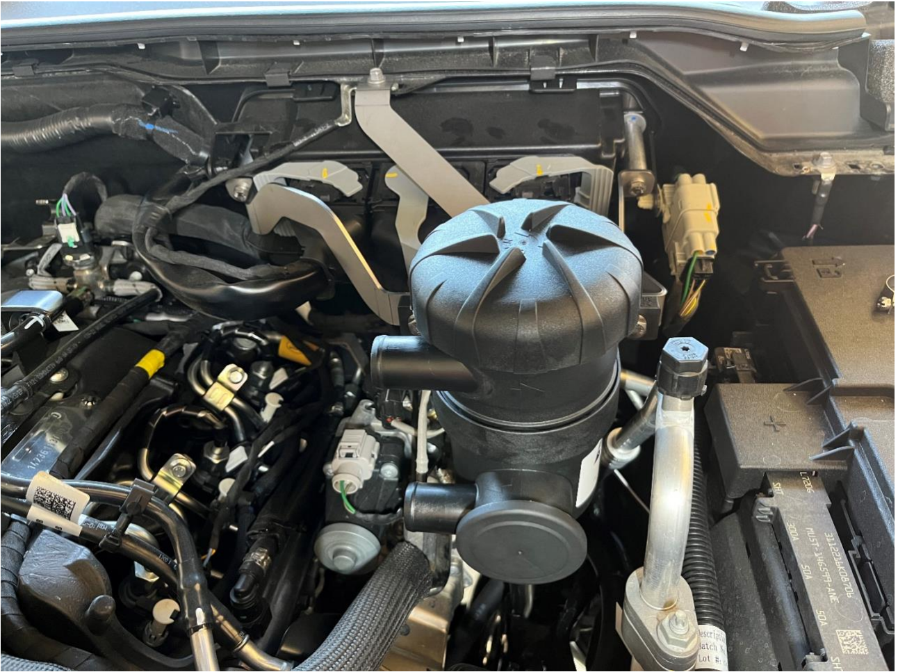
ProVent 200 bolted to bracket– Please note ProVent rotation in this image is correct, refer to the image on the last page of this installation guide for how to rotate the unit.
