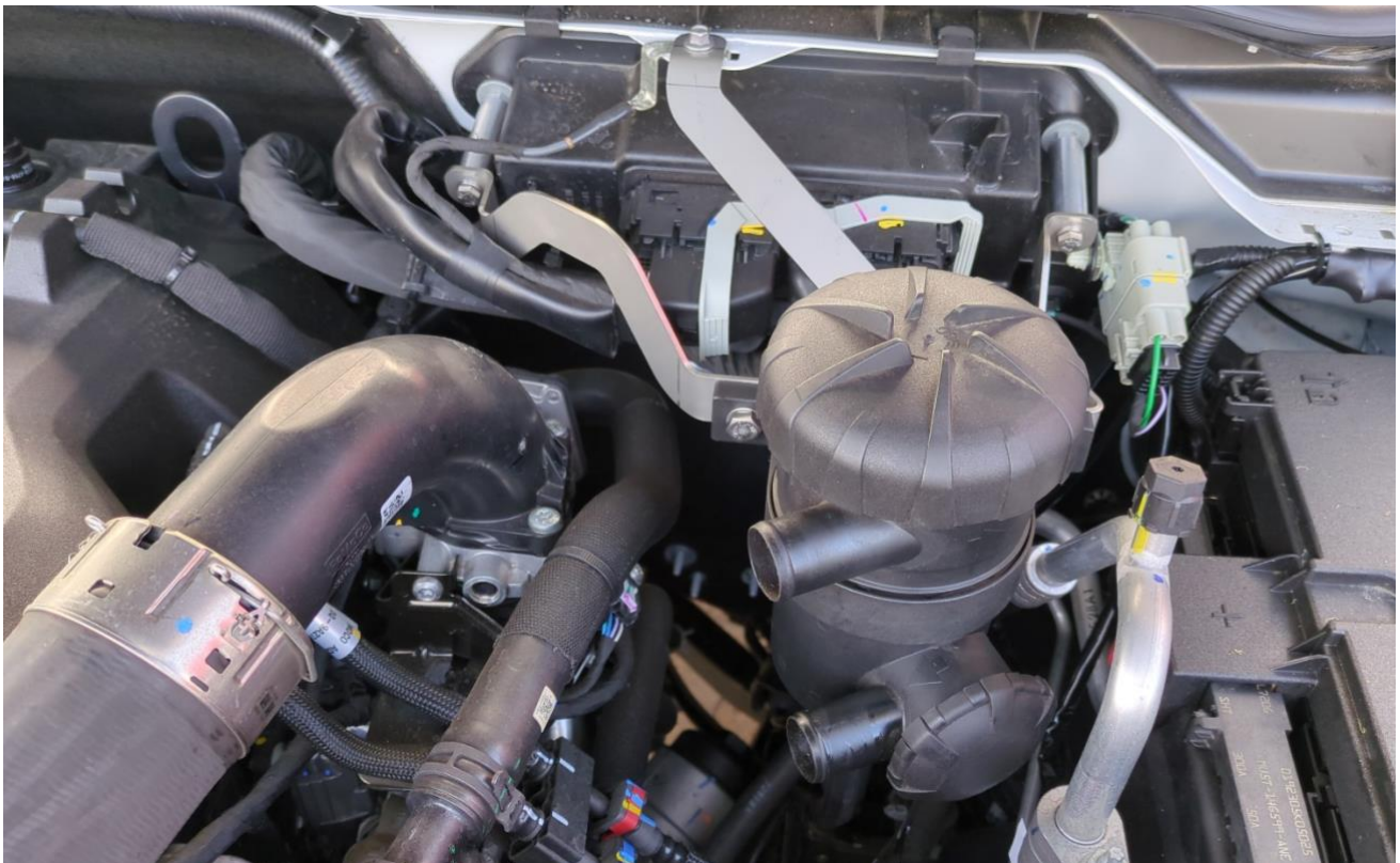
ProVent 200 bolted to bracket— Please note ProVent rotation in this image is correct, refer to the image on the last page of this installation guide for how to rotate the unit.
