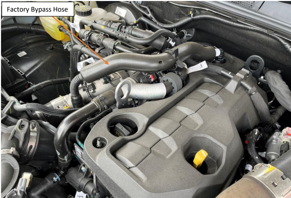
Factory bypass hose location
