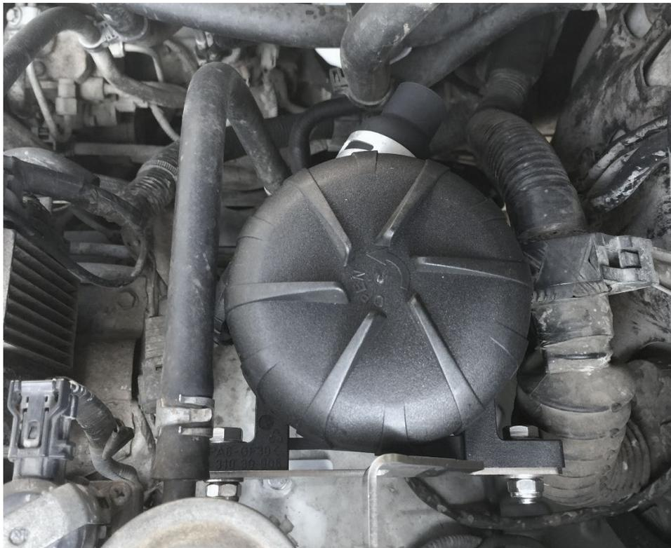
*ProVent bolted in place at correct rotation.*
