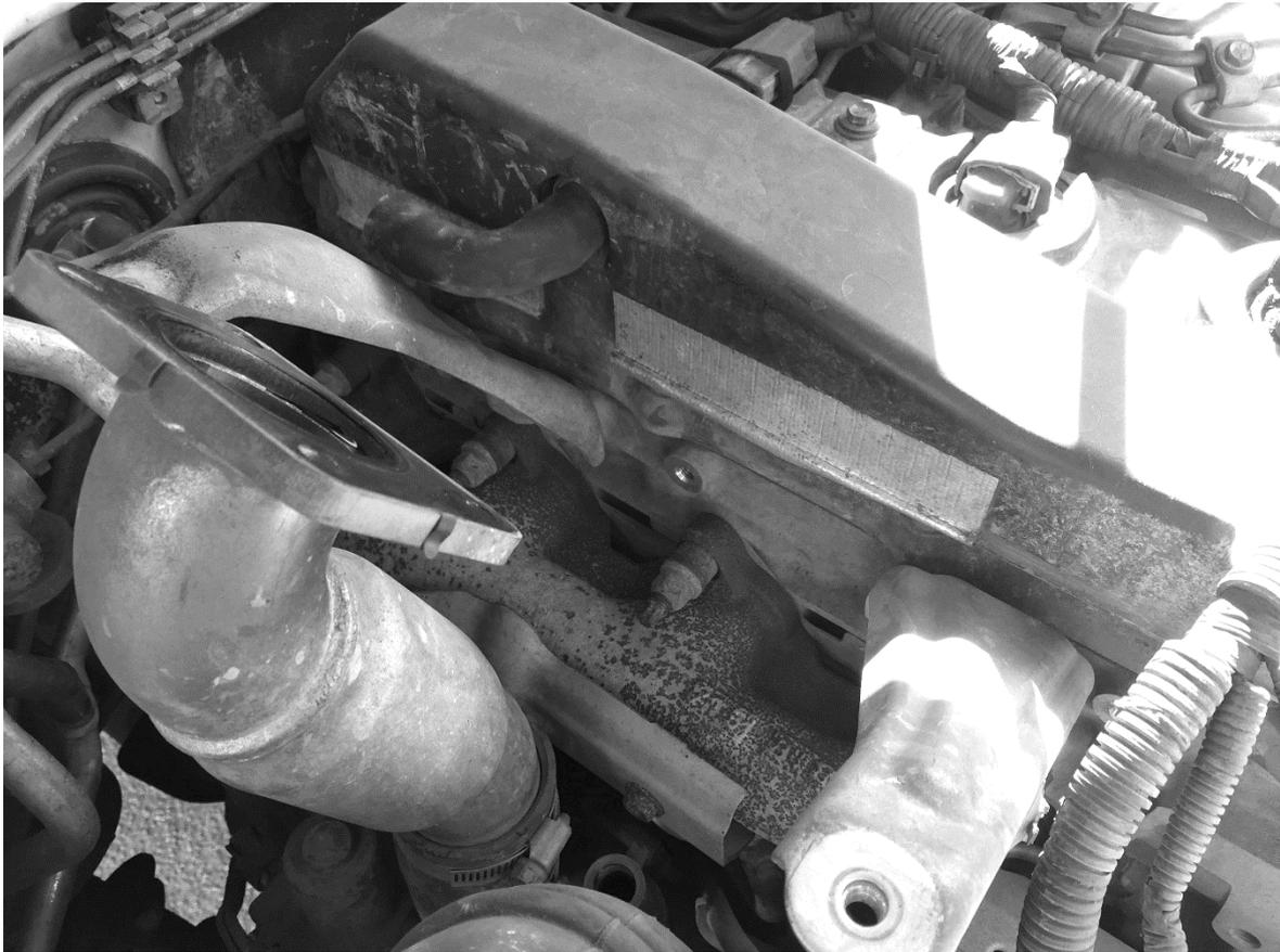
*Image shows factory intercooler removed, factory bypass hose removed, and rubber elbow reinstalled facing towards the rear of the vehicle*
