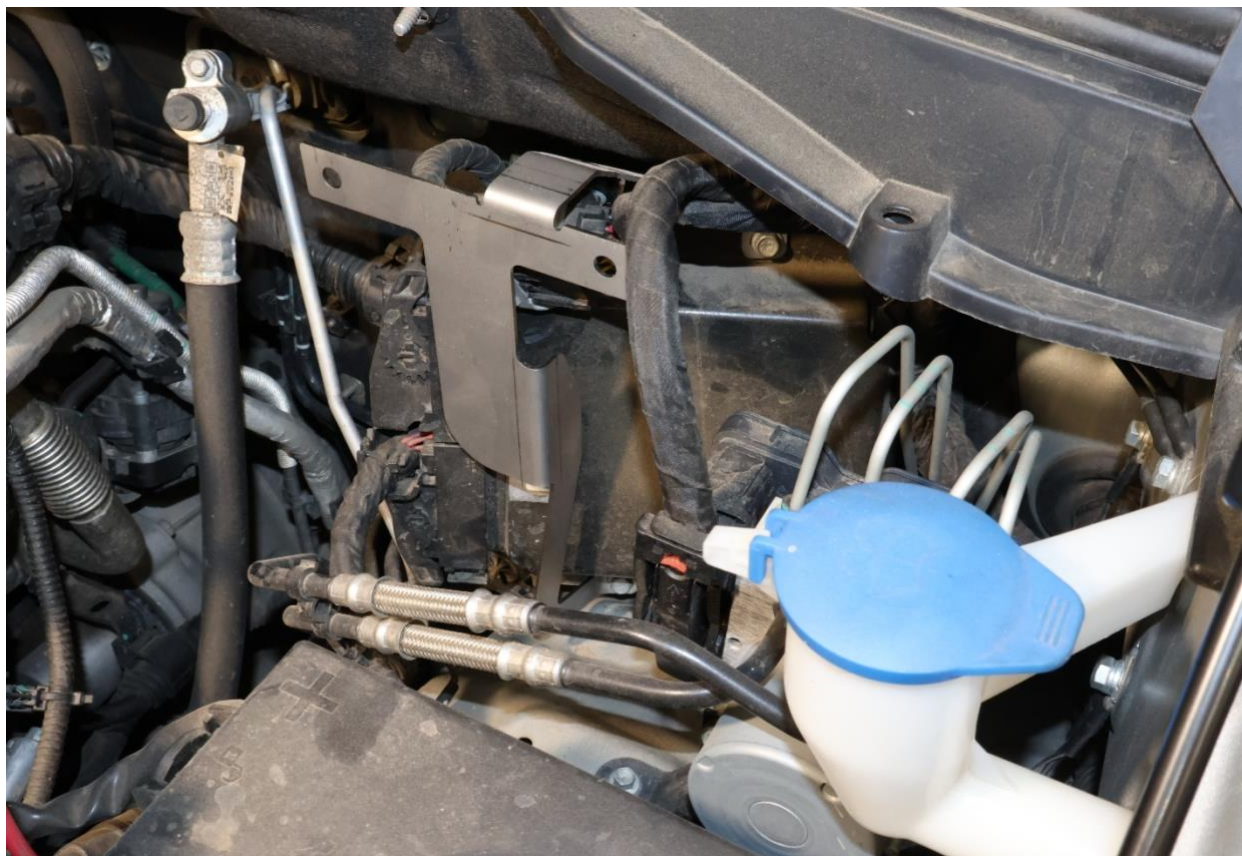
Great Wall Cannon Engine Bay ProVent Bracket Mounted in Place
