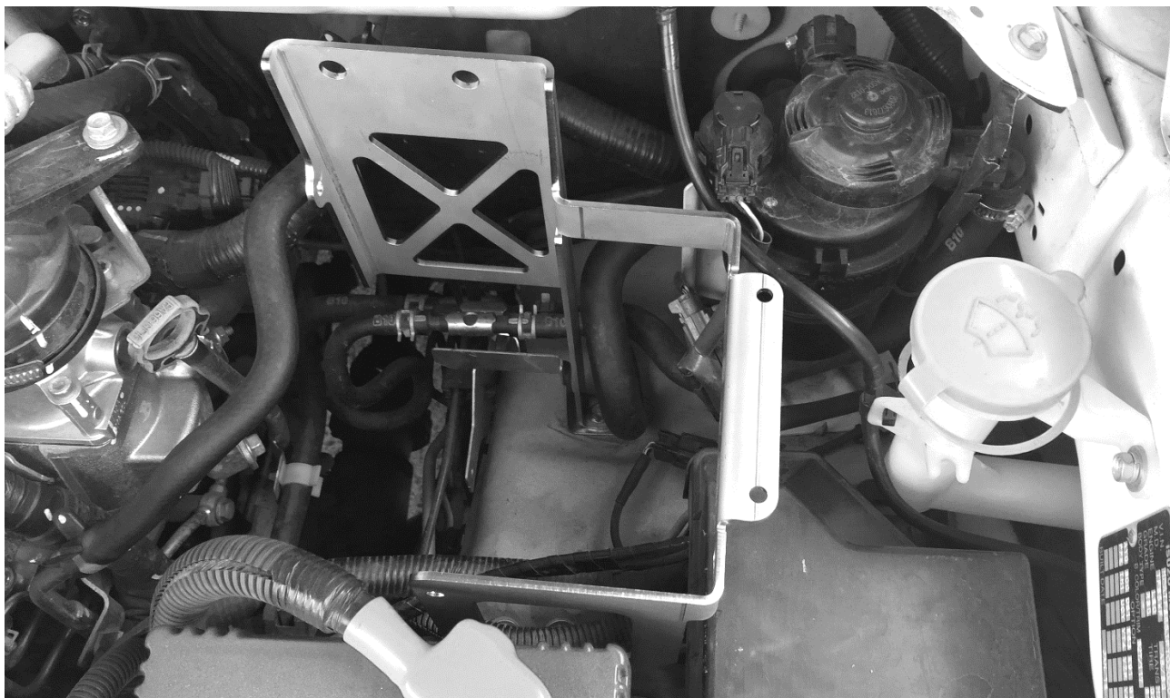
D-Max Engine Bay- Rear Passenger Side with new bracket installed
