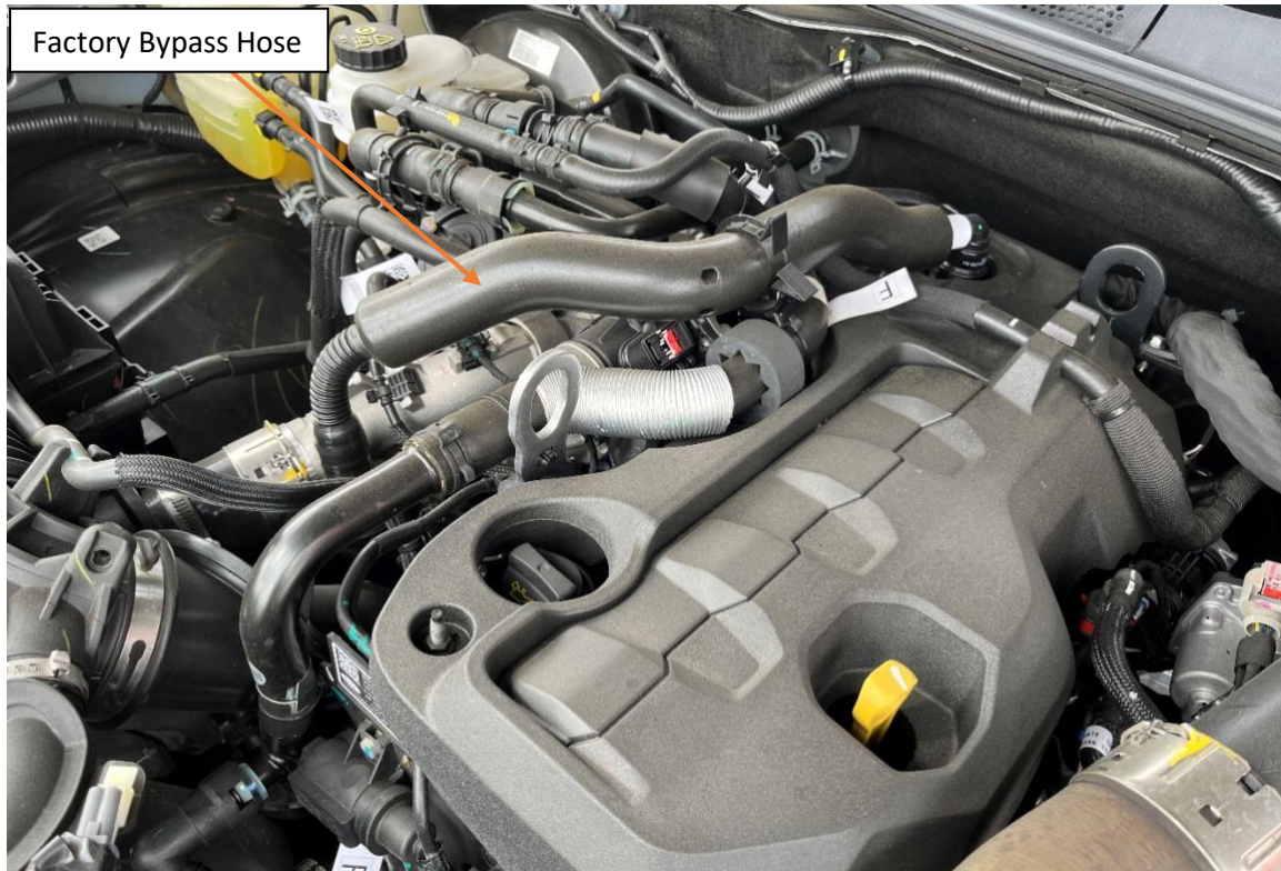
Factory bypass hose location
