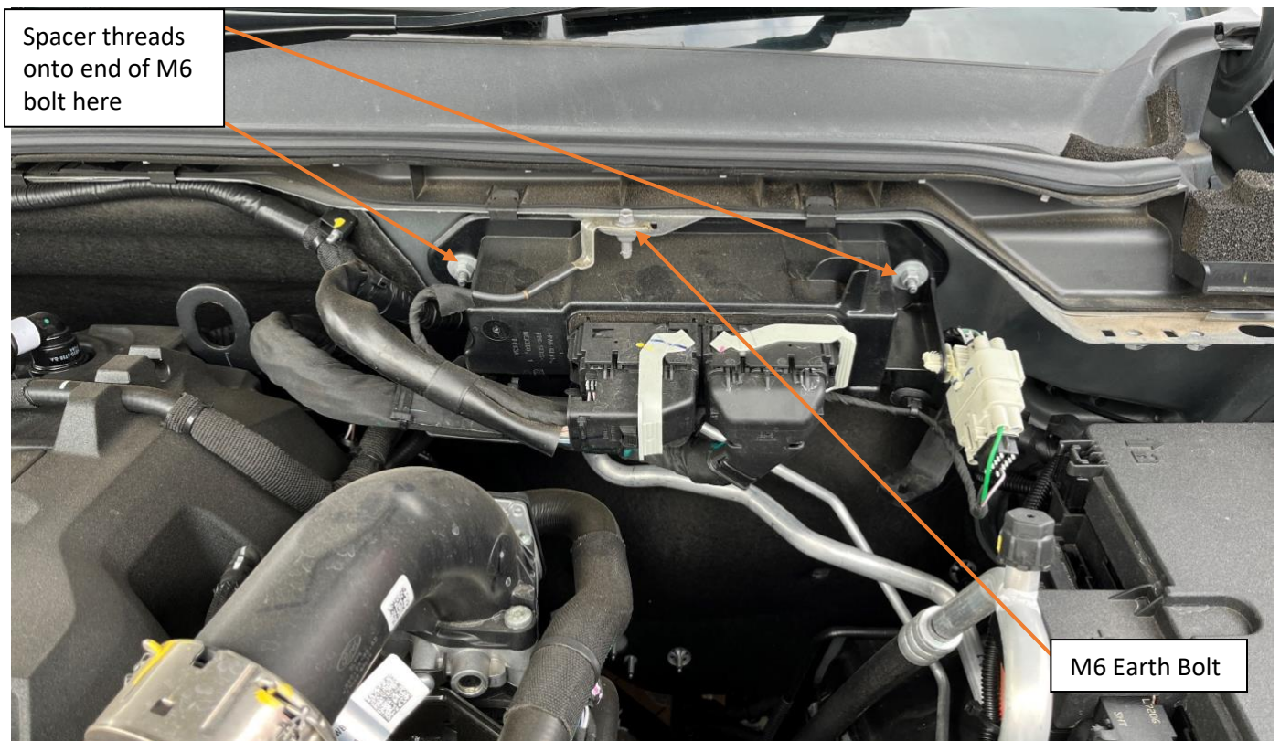
Location of alloy spacer mounting
