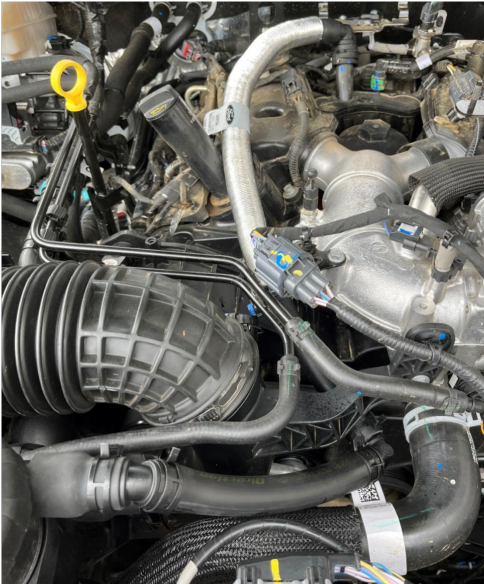
ProVent Ultimate Catch Can Supply Line Installed
