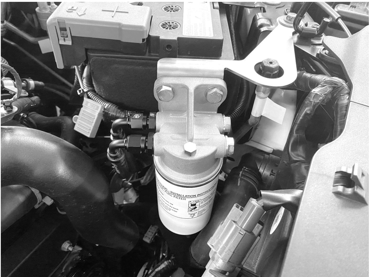
Fuel hose routing for pre-filter on Ranger 2022+
