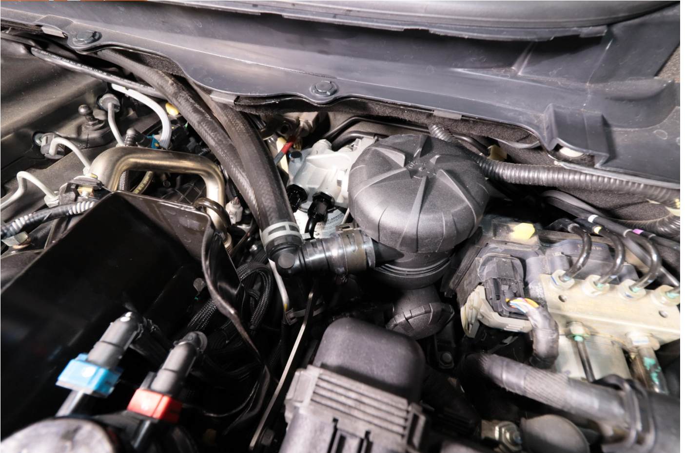
Completed installation of the ProVent® and PL150DP
