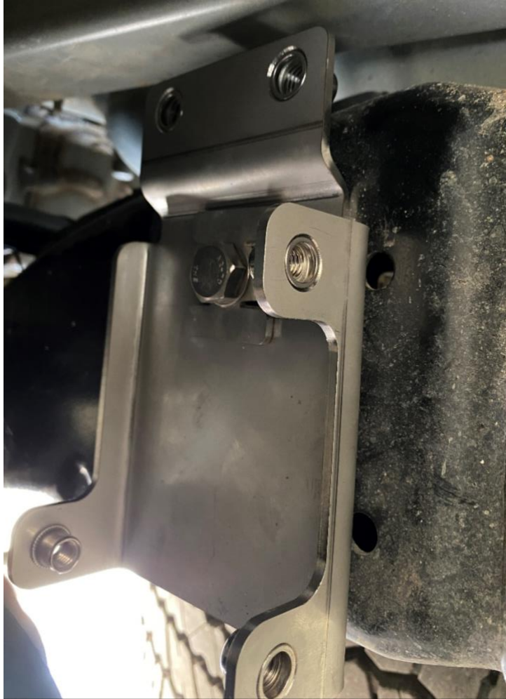
PreLine-Plus bracket secured in place, note how smaller bracket lock in to prevent movement from the main bracket
