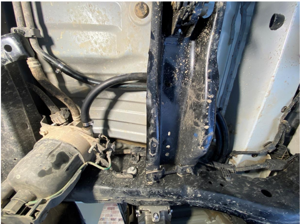
Fuel hose routing for PreLine-Plus on LC300
