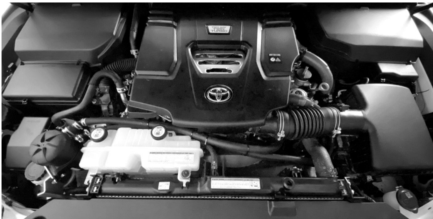
Hose configuration in Land Cruiser 300 Series with ProVent Ultimate Catch Can kit installed
