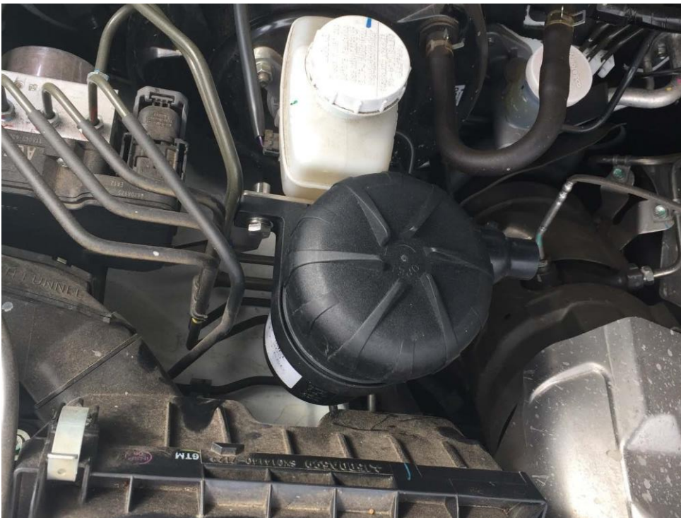
MQ Triton: ProVent® 200 bolted in place on mounting bracket. PLPV629DPC COMBO KIT
