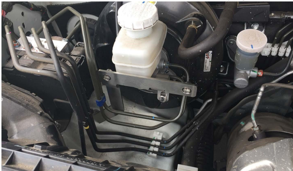
MQ Triton: ProVent® 200 mounting bracket in place.
