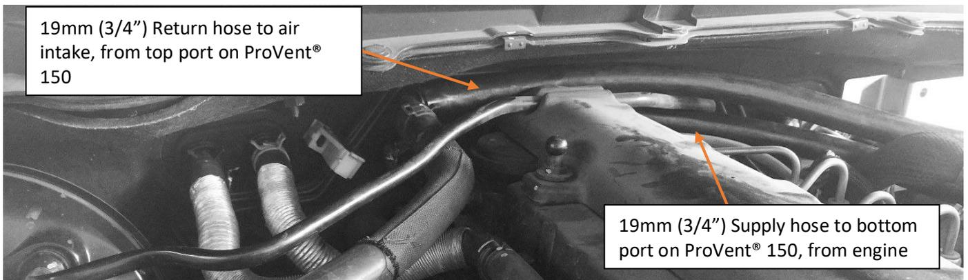
*Hose configuration in PX Ranger with ProVent® 150 installed – Note, the hose to the ProVent® need to be run underneath the hard pipe in order to fit the engine cover back on, the hoses are long enough to allow for this. (hose clamps not shown)*
