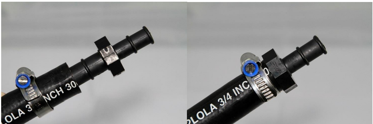
19mm end of hose joiner inserted into 19mm Hose and secured with 20-32mm worm drive clamp
