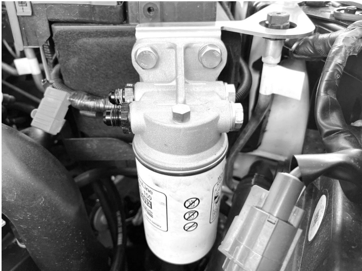
PreLine 150 in place on bracket with M16x1.5 to -6 Adaptors installed
