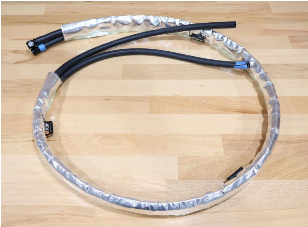
Fuel hoses inside of heat sleeve, tape used for identification to ensure correct port orientation of hoses
