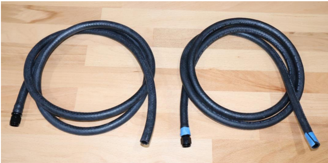
Picture of fuel hose with fittings– Note tape used to mark one of the hoses at both ends
