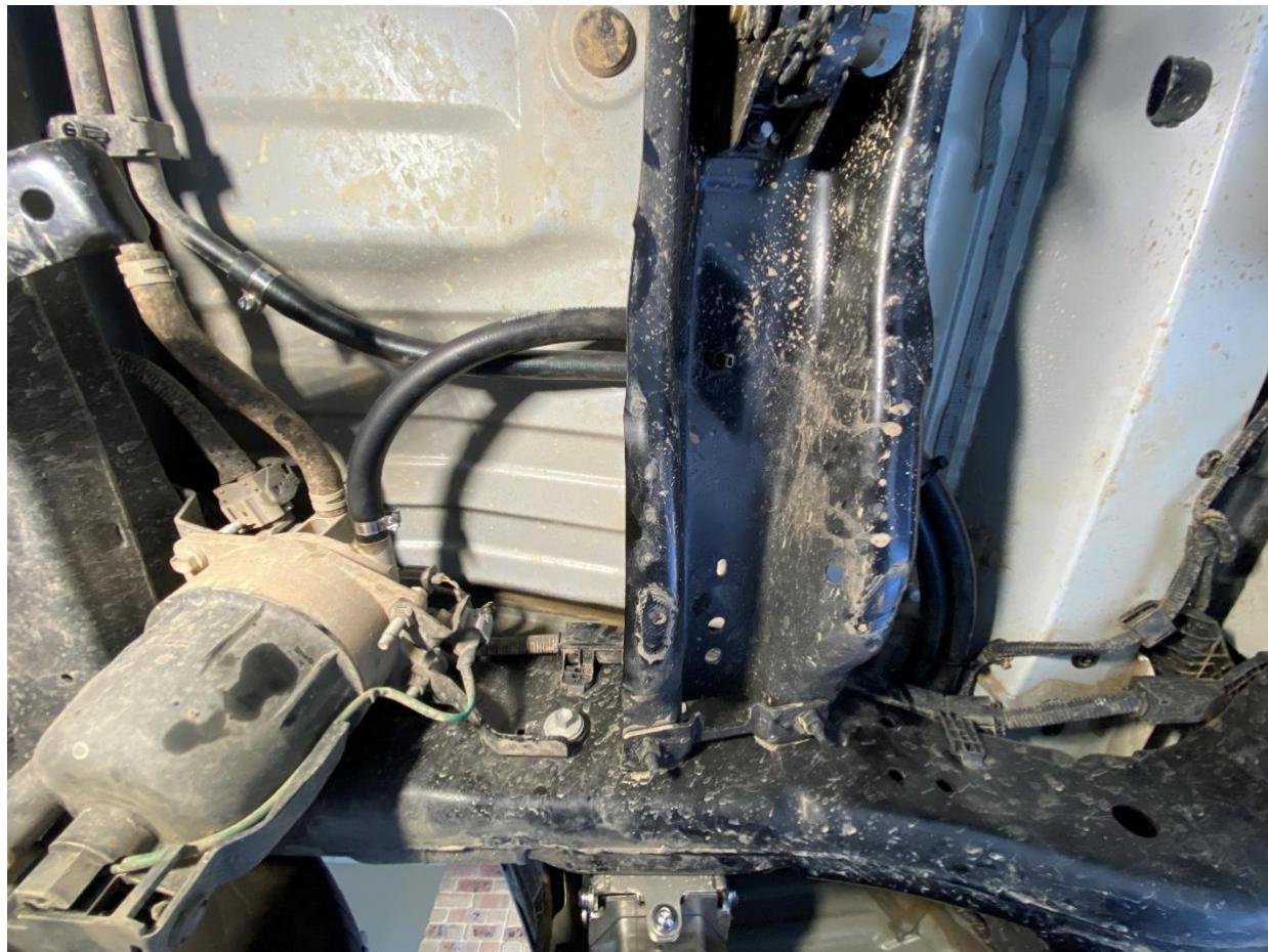
Fuel hose routing for PreLine-Plus on LC300
