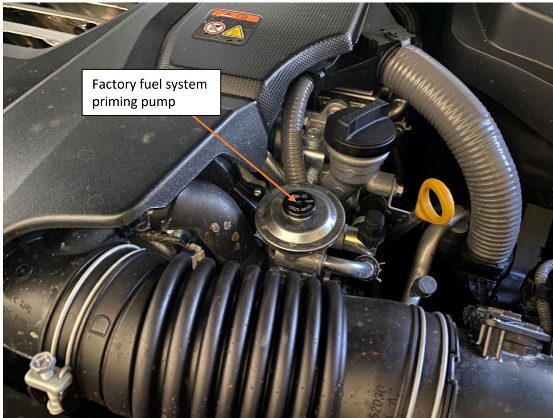
LC300 factory fuel system priming pump
