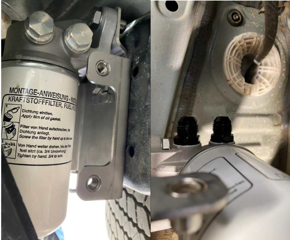
PreLine-Plus in place on bracket with M16x1.5 to -8 Adaptors installed
