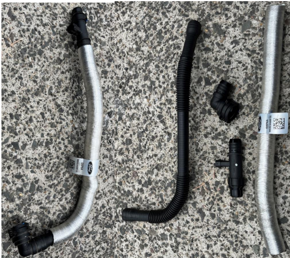
Factory bypass hose after disassembly
