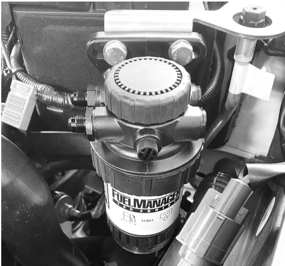
Fuel Manager in place on bracket with M16x1.5 to -6 Adaptors and Plugs installed
