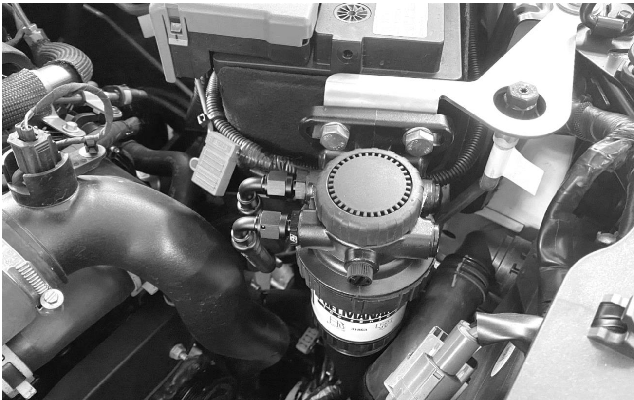
Fuel hose routing for Post-filter on Ranger 2022+
