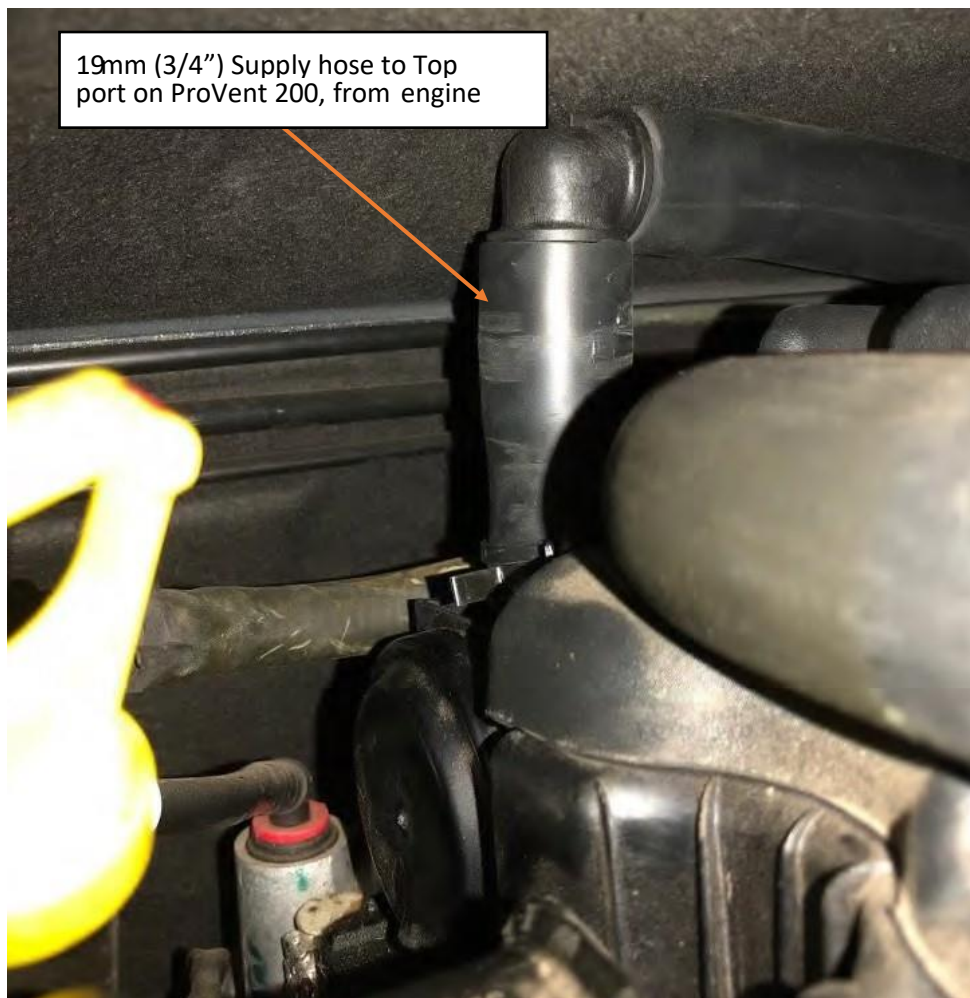
Engine cover connection to ProVent Upper port
