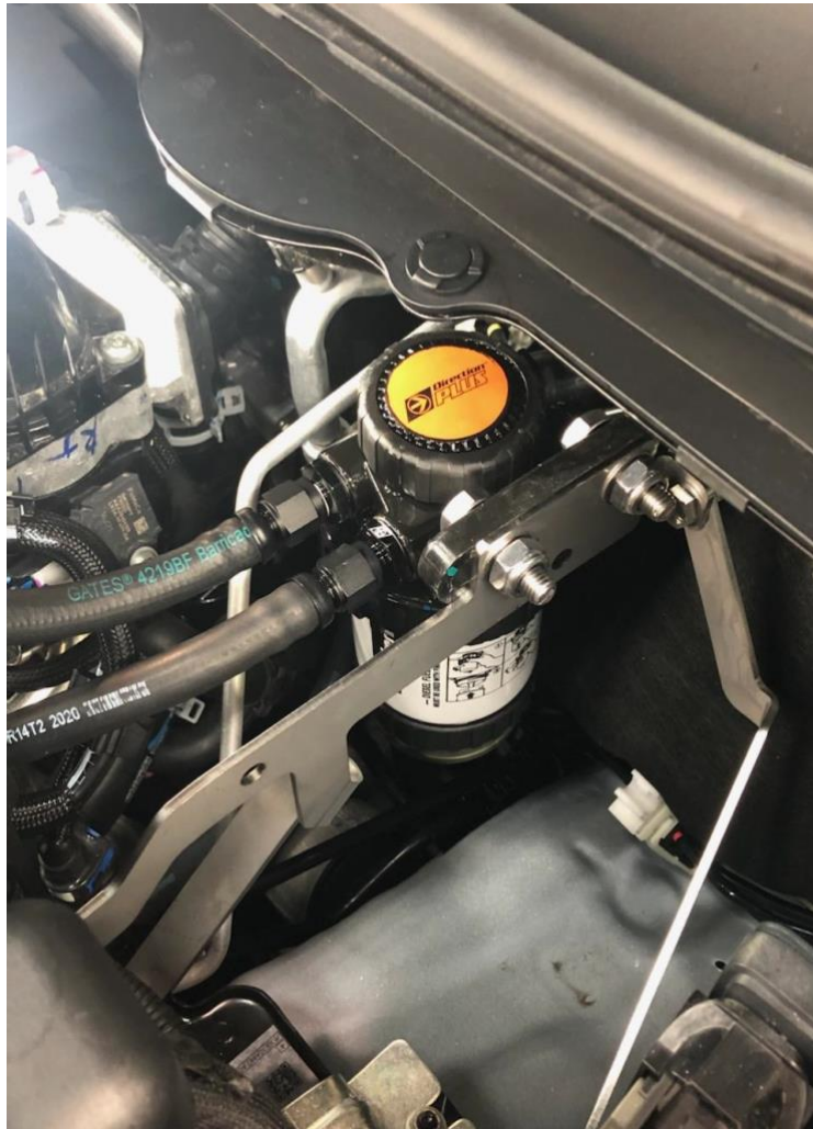
Completed installation of the Fuel Manager POST-FILTER PF664DPK
