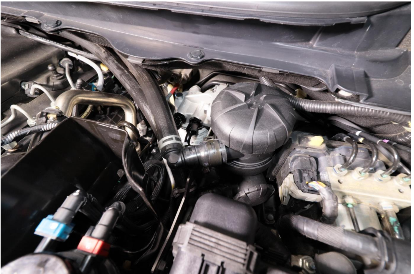
Completed installation of the ProVent Ultimate Catch Can and Post-filter Kit
