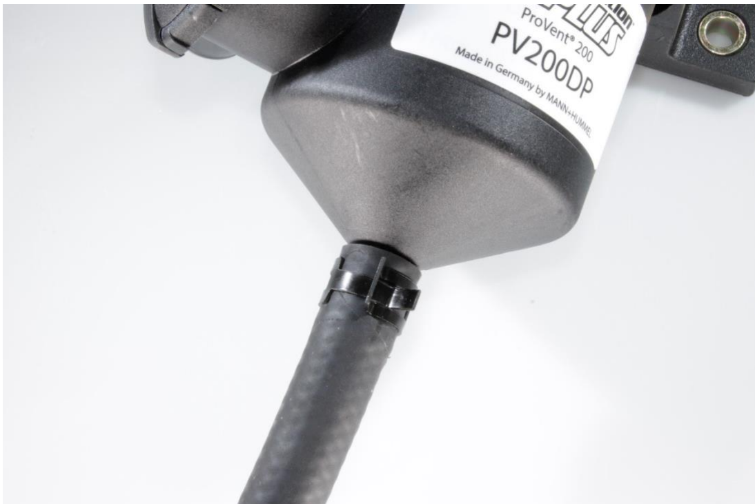
Provent® 200 with 12mm hose connected and secured with 12mm spring clamp
