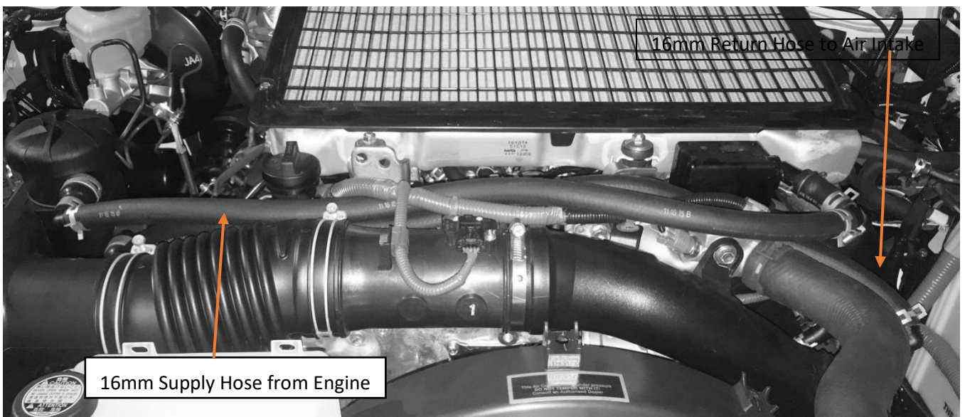
Engine bay hose locations for Land Cruiser 70 series V8 diesel
