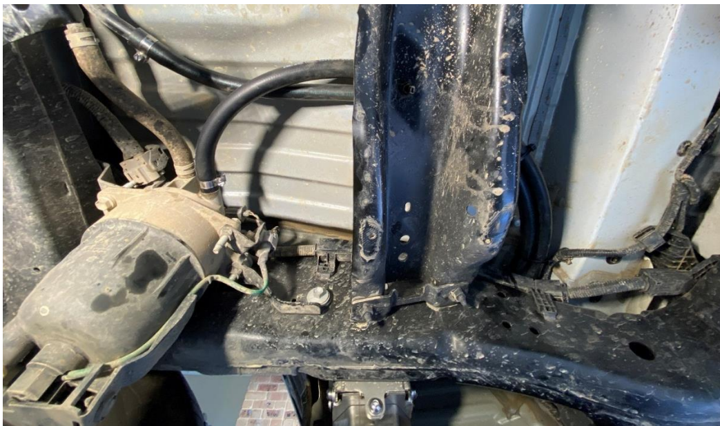
Fuel hose routing for Fuel Manager pre-filter on LC300
