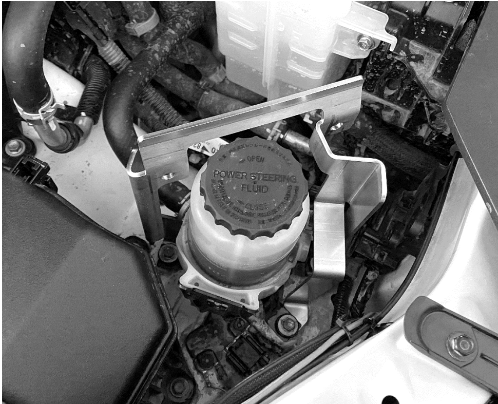
New Provent Ultimate Catch Can bracket mounted in place, reuse original bolts
