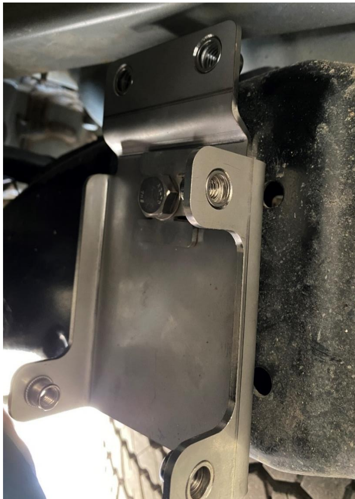
Fuel Manager bracket secured in place, note how smaller bracket lock in to prevent movement from the main bracket
