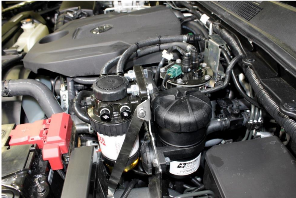
Completed installation of both the Post-Filter and ProVent
