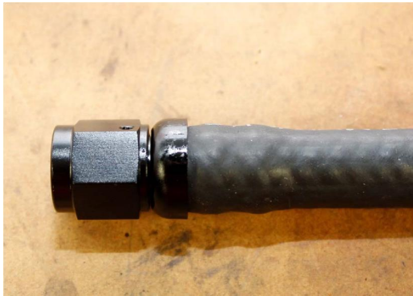
Correctly installed push lock fitting
