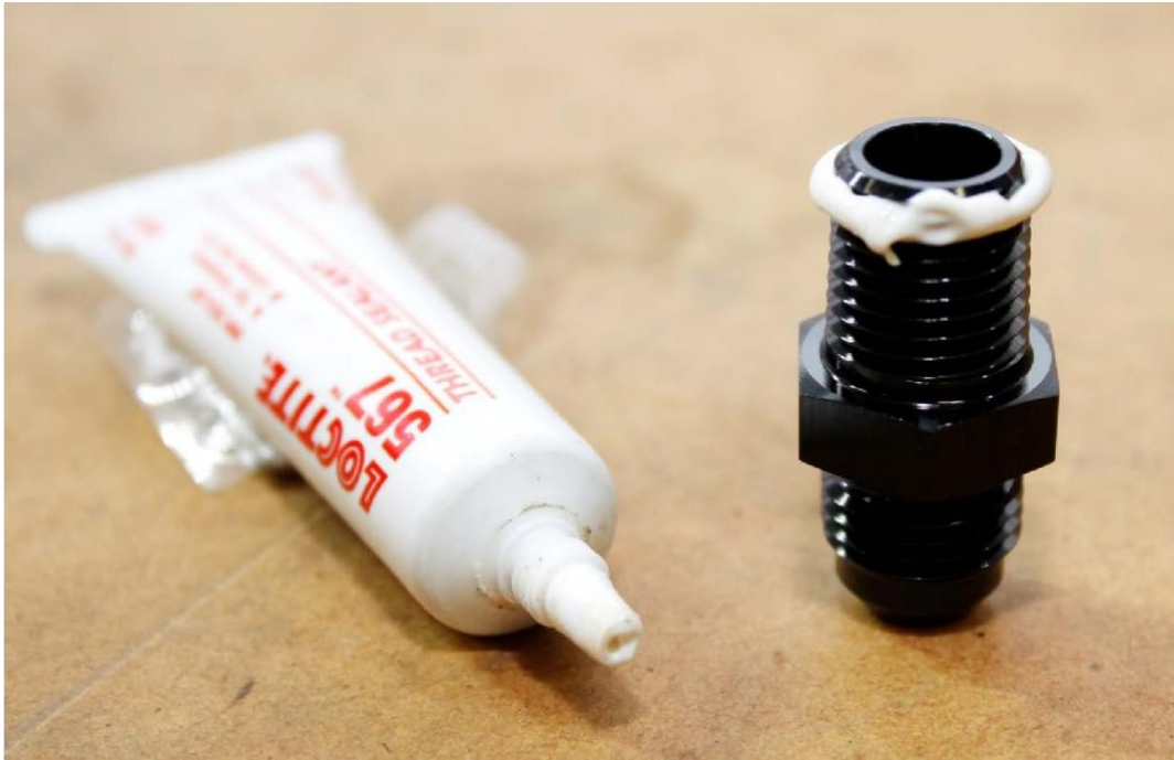
Fitting with Loctite applied
