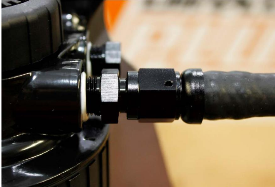
Push lock fitting connected to the Post-Filter head
