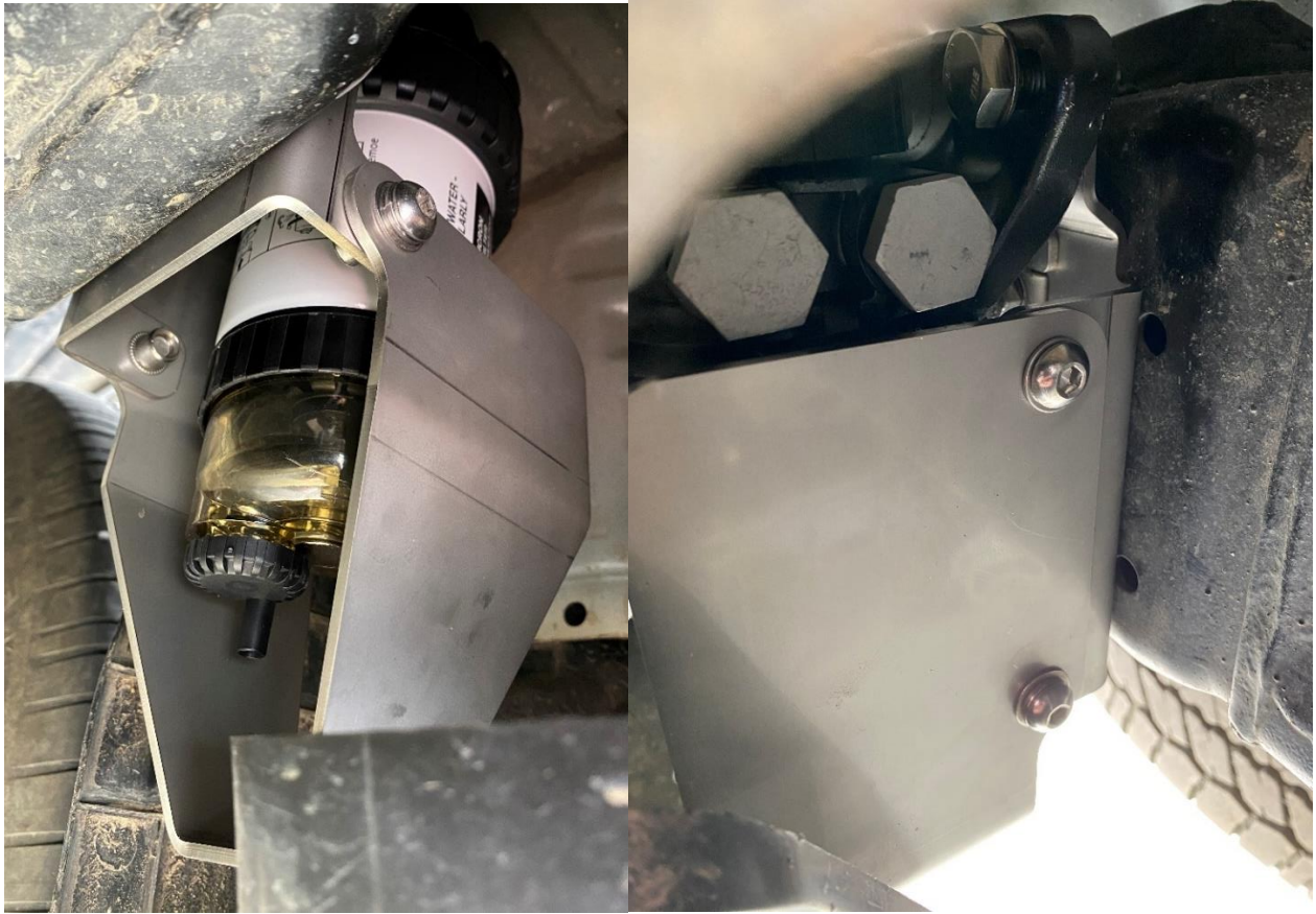
Fuel Manager filter cover (LC300FM1000.3) bolted in place
