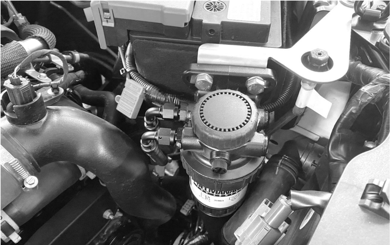
Fuel hose routing for pre-filter on Ranger 2022+
