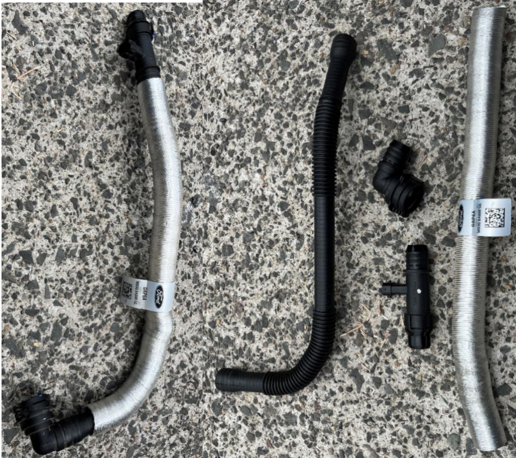
Factory bypass hose after disassembly
