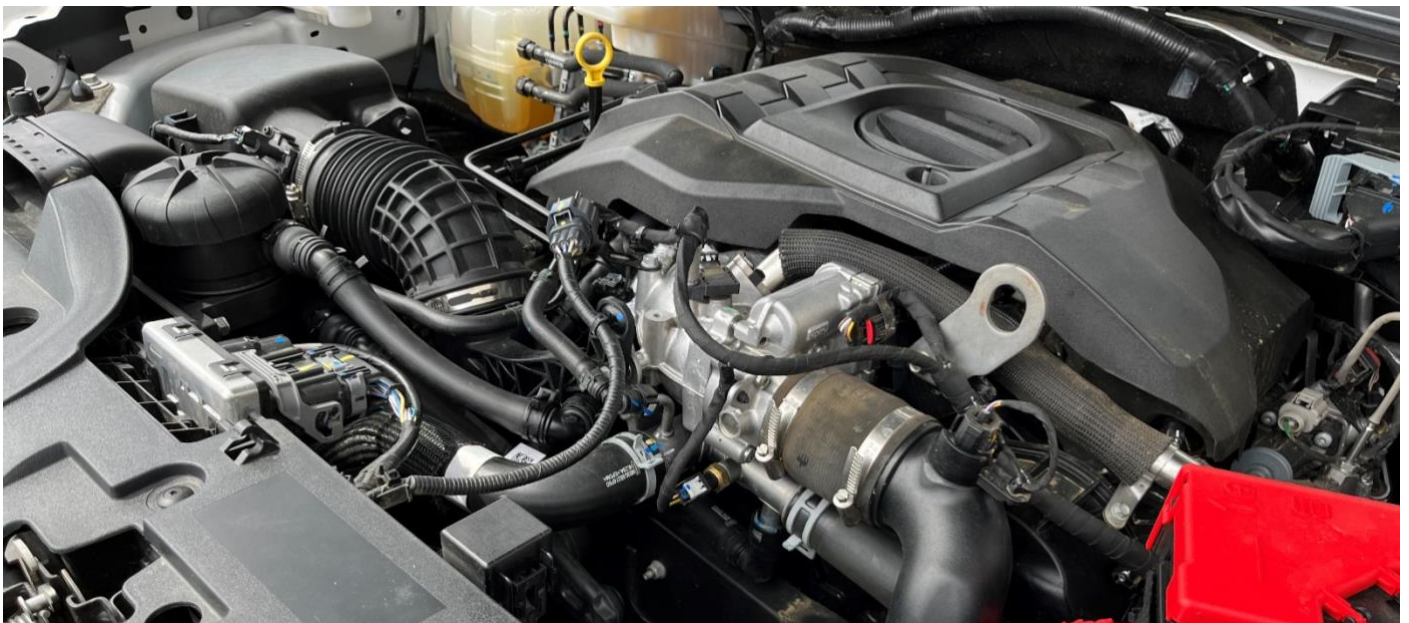
Finished Install – Check to make sure everything is secure and then put the engine cover and radiator cowl panel back on
