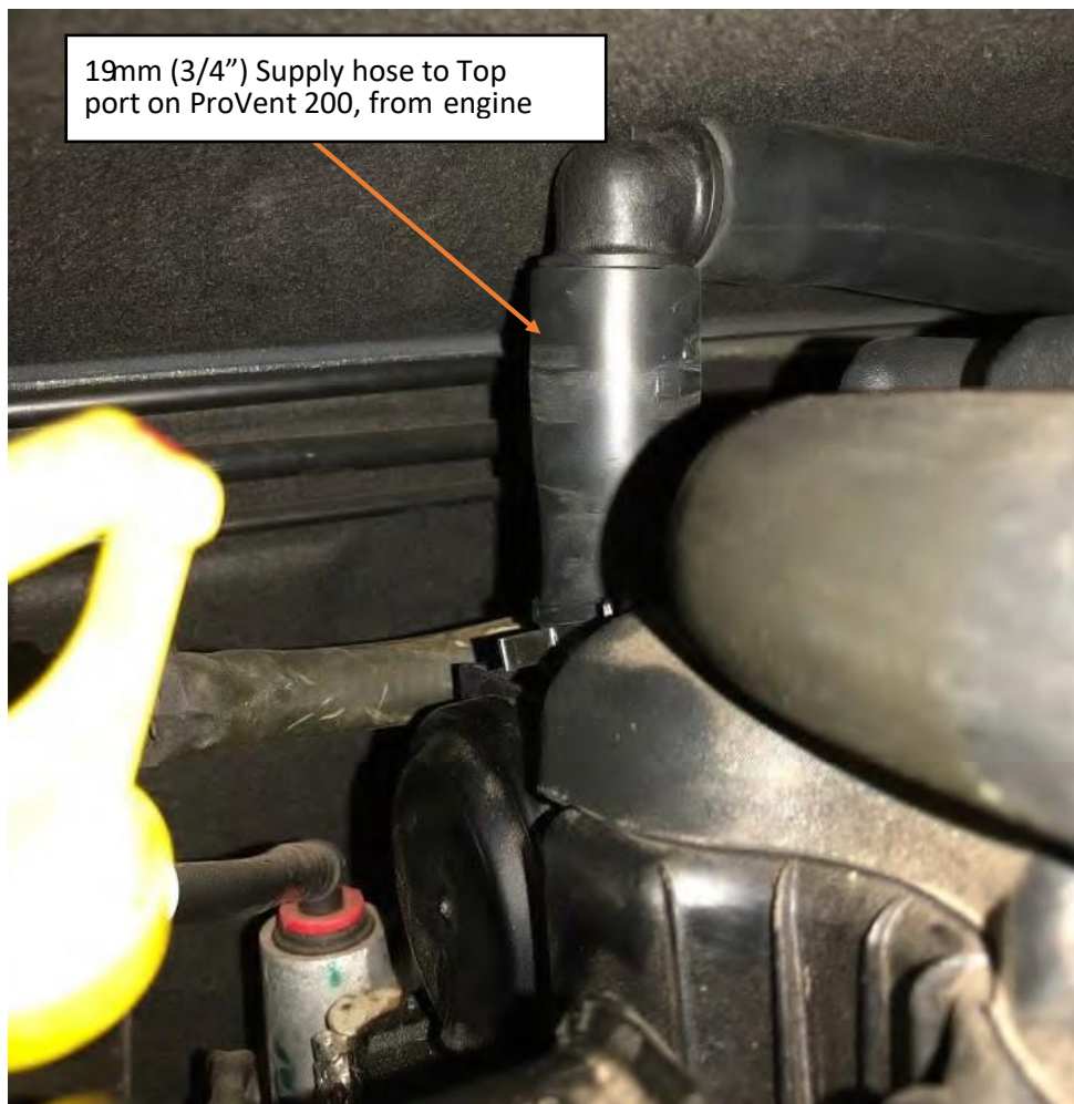
Engine cover connection to ProVent Upper port
