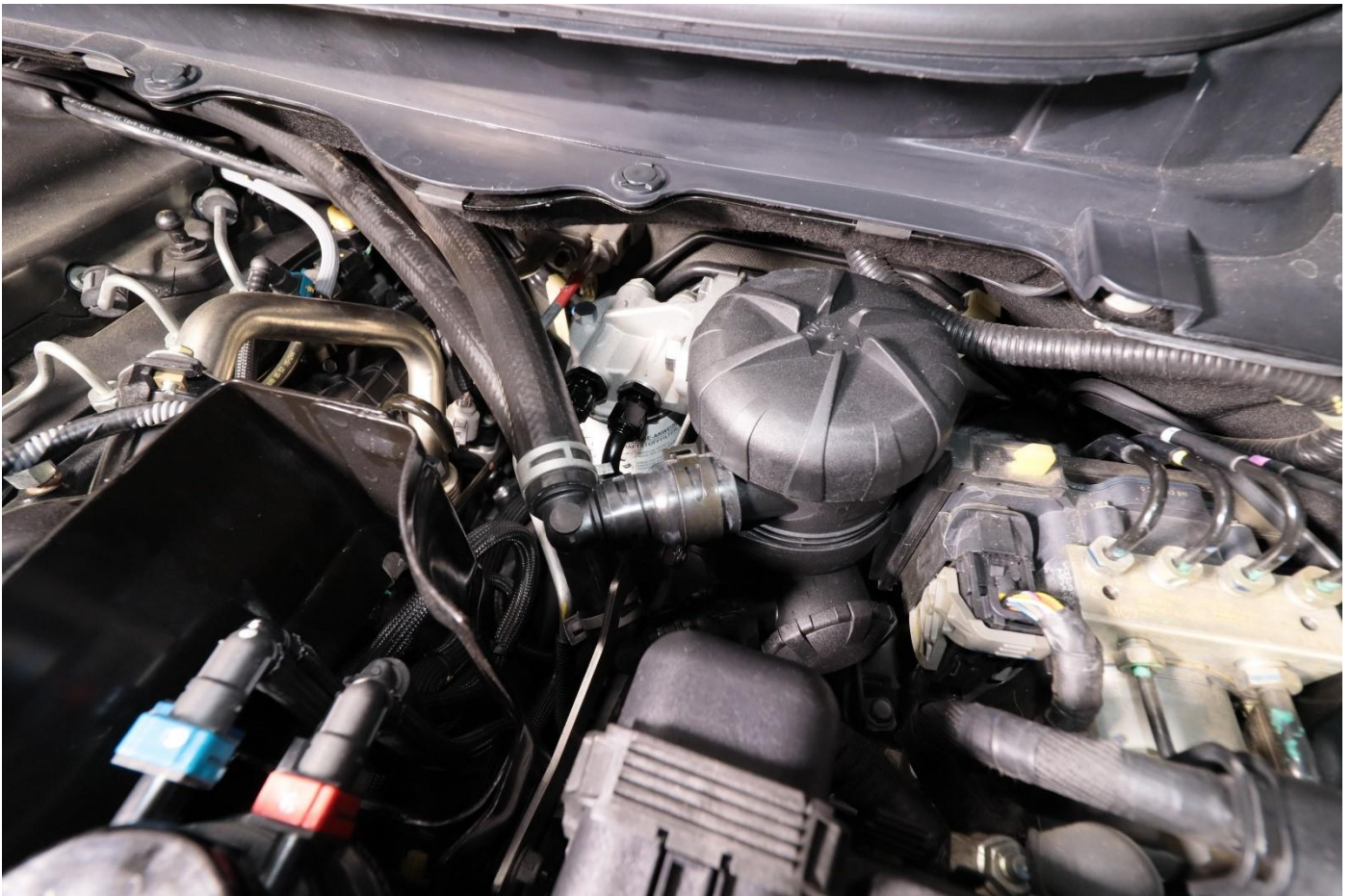
Completed installation of the ProVent® and Pre-filter Kit
