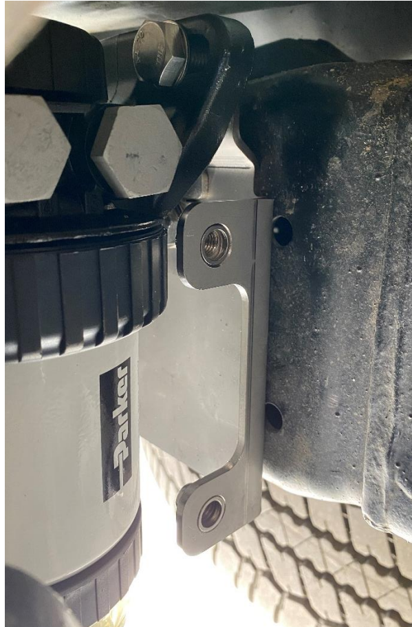
Fuel Manager Pre-Filter in place on bracket, fuel fittings face rear of vehicle
