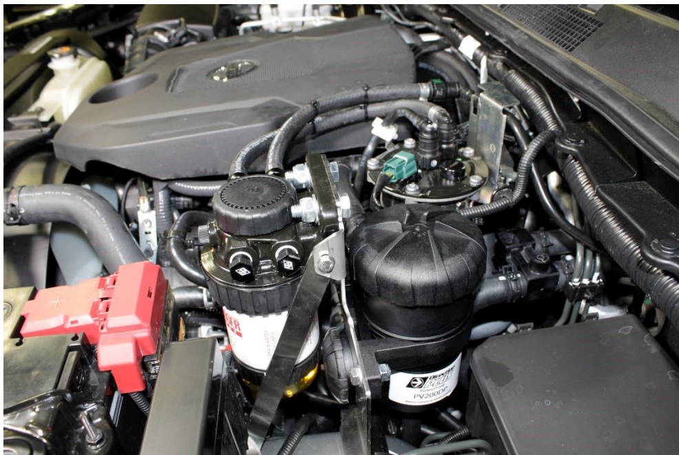
Completed installation of both the Pre-Filter and ProVent
