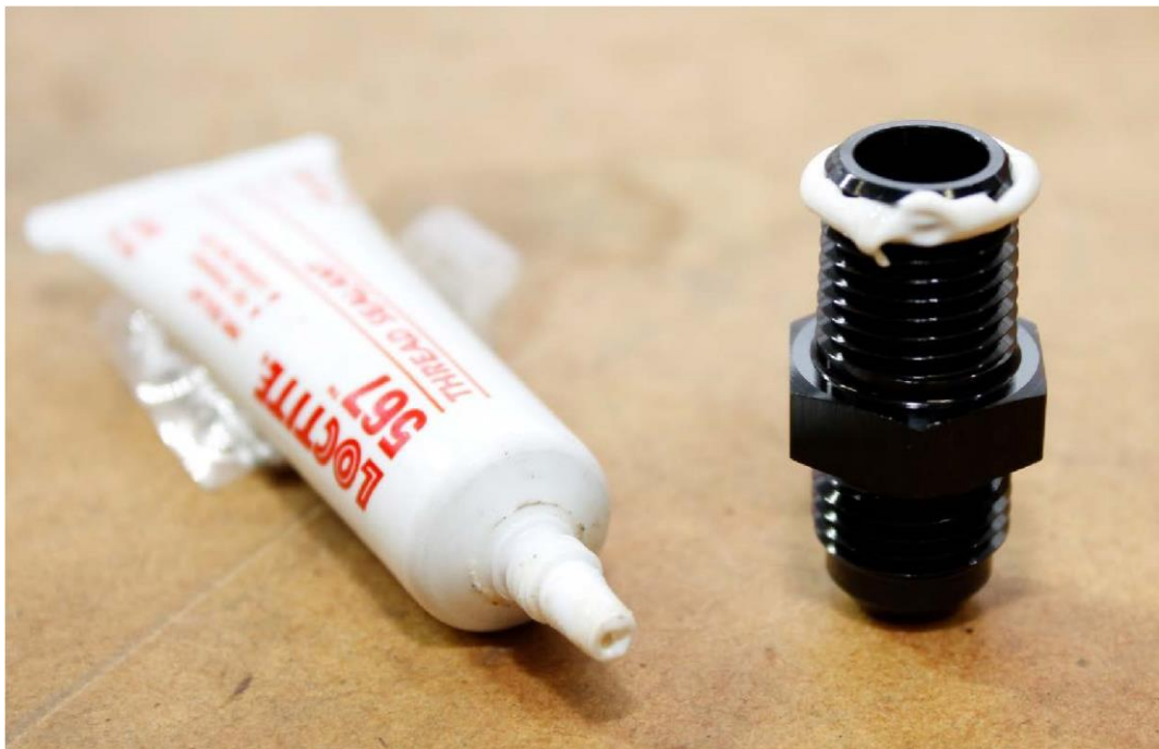
Fitting with Loctite applied
