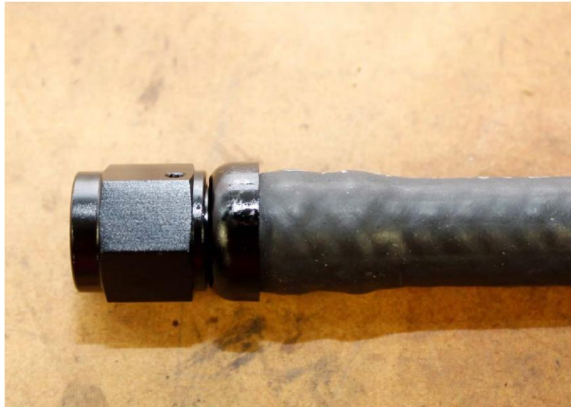
Correctly installed push lock fitting
