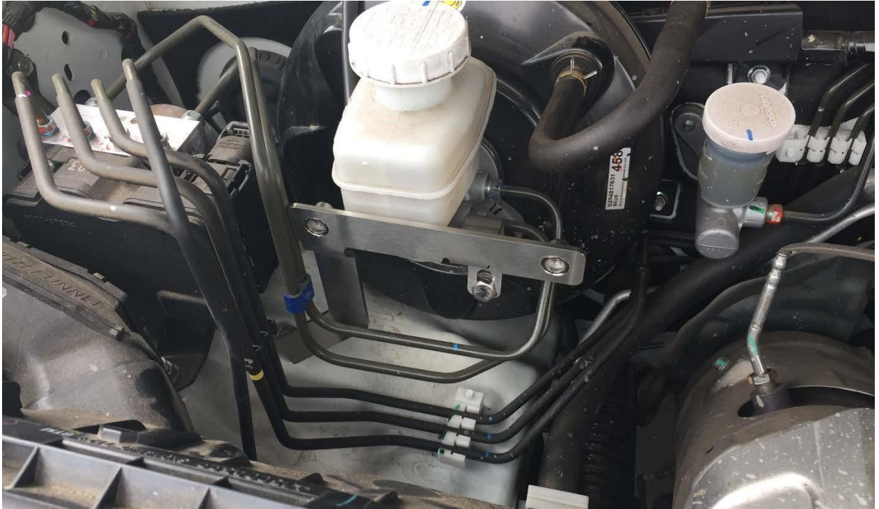
MQ Triton: ProVent® 200 mounting bracket in place.
