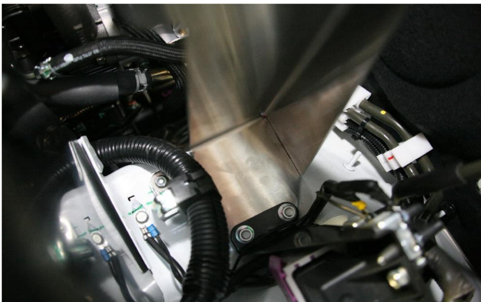
mounting bracket installed
