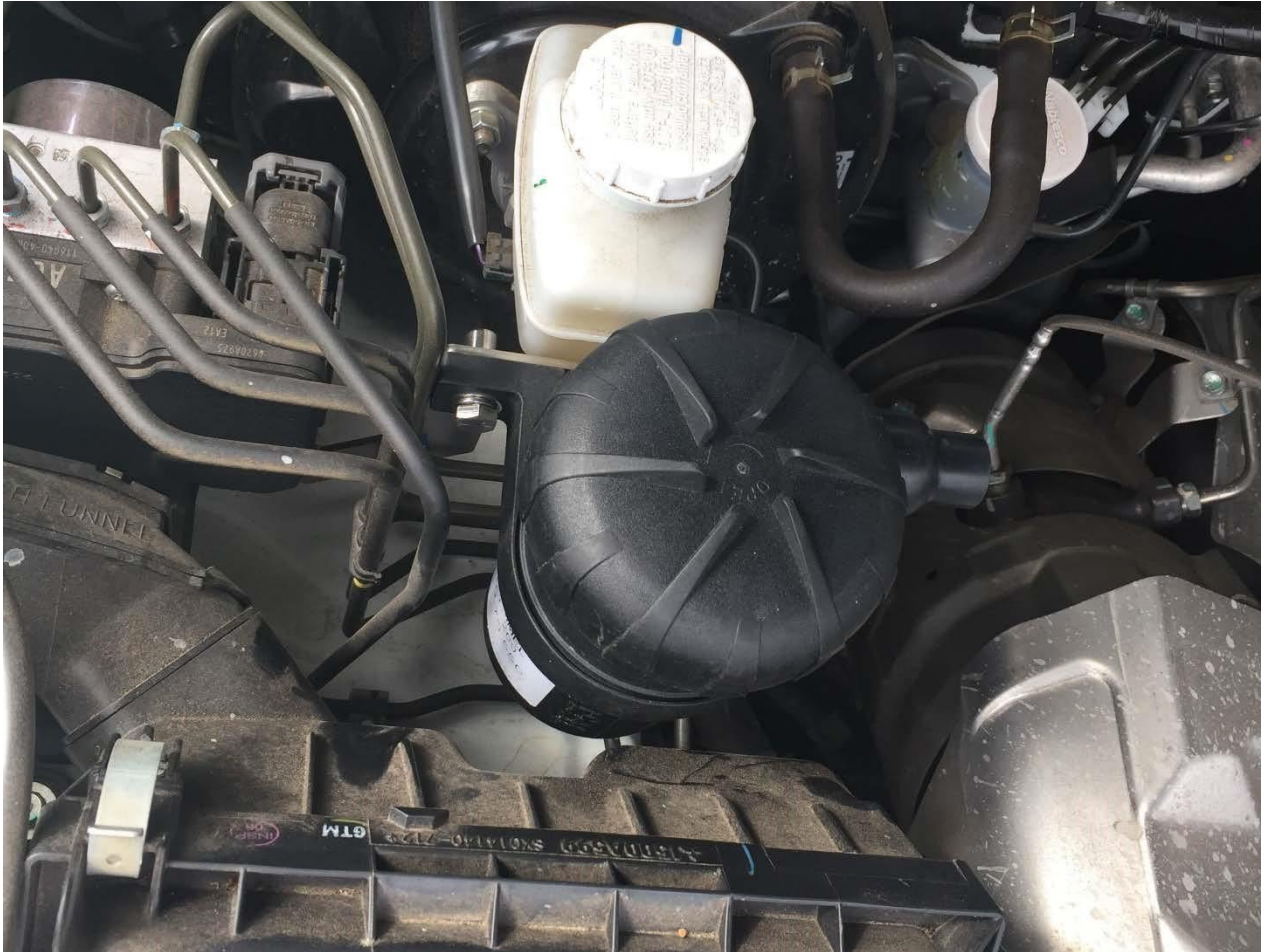
MQ Triton: ProVent® 200 bolted in place on mounting bracket.
