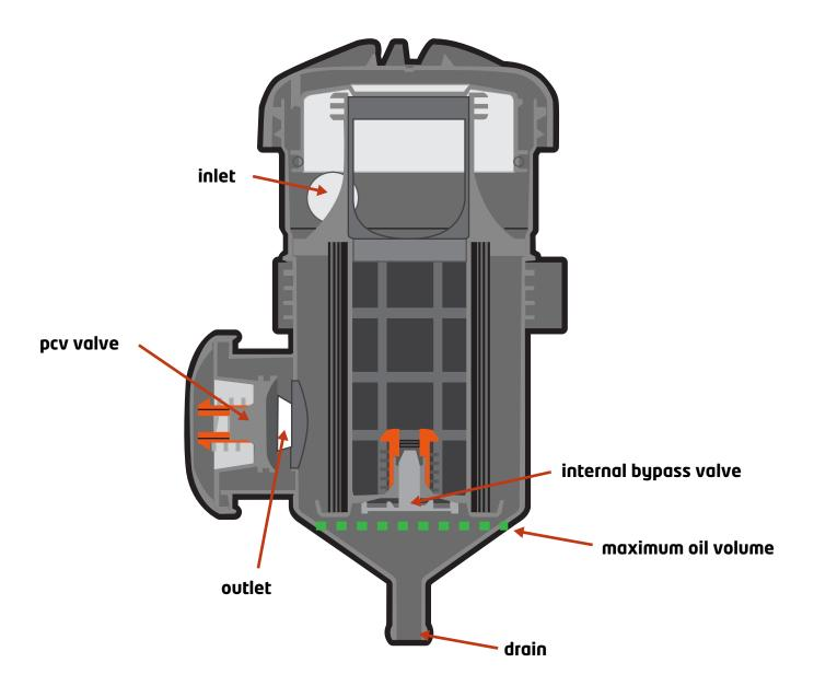
Due to the way the internally vented PV200 works, the PV200 must be drained regularly to ensure correct operation of the internal bypass valve. Failure to regularly draining/servicing the Catch Can may cause engine damage due to over pressurisation of the crankcase ventilation system.
