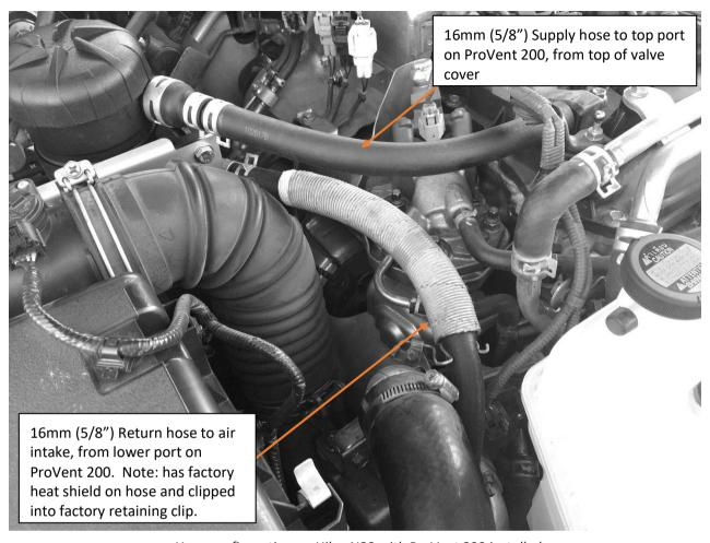
Hose configuration on Hilux N80 with ProVent 200 installed
